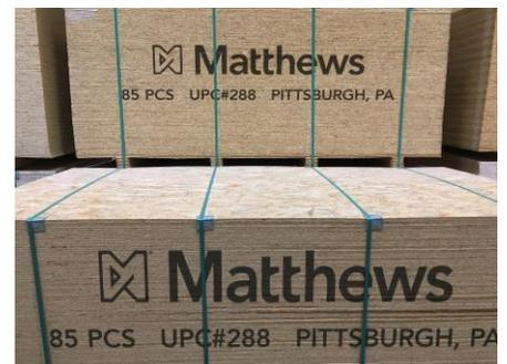
Matthews is a key supplier of marking and coding equipment to the wood industry. The valve jet printers they're known for can withstand the harsh environment of the wood mills and require
